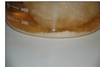
Precipitates also rain out onto the bottom of the beaker.
