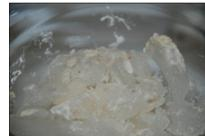
Preparing samples: Ice is placed in beakers and allowed to evaporate in a clean environment. Precipitates form on top of the ice as it melts.
