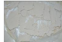
Once the solution has nearly evaporated, the mixture is poured onto wax paper covered trays and allowed to dry and ground into powder.
