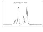
Identifying elemental compounds with the Spherical Grating Monochromator. We found very specific signatures for Calcium. Our samples (left) match the spectrum for calcium carbonate (CaCO<sub>3</sub>) as illustrated on the right from Nafisi et al. 2001.
