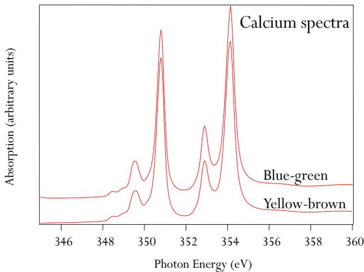
Figure 13. Calcium eV range TEY spectrums of both types of ice from Bosworth Creek. These signatures closely resemble a CaCo<sub>3</sub> spectrum (From Ko et al. 2007) and are assumed to be calcium carbonate.
