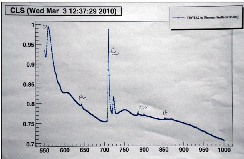
Figure 15a. The TEY spectrum for oxygen in soil is a typical signature occurring near the 550 eV range. Other elements occurring in this sequence include manganese, iron, cobalt and nickel.
